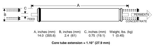
Notice: Minimum permeate flow for individual elements is 28 percent below listed flow. All membrane elements are supplied with a brine seal and o-rings. Most elements are packaged dry, sealed in a polyethylene bags, and shipped in a cardboard box. Some elements are sealed in polyethylene bags containing less than 1.0% sodium meta-bisulfite solution and shipped in a cardboard box.
