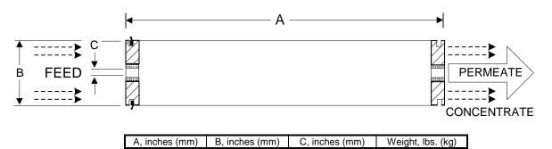
Notice: Permeate flow for individual elements may vary -20/+25 percent. Membrane active area may vary +/-4%. Element weight may vary. All membrane elements are supplied with a brine seal, interconnector, and o-rings. Elements are enclosed in a sealed polyethylene bag containing less than 1.0% sodium meta-bisulfite solution, and then packaged in a cardboard box.
