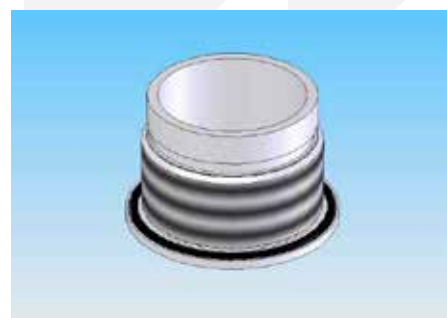
Threaded side port; seal seating on side port
